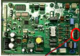
Unplug pump from board (maroon colored connector with 1 white and 1 yellow wire)
