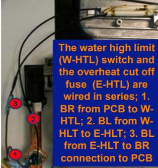
The water high limit (W-HTL) switch and the overheat cut off fuse (E-HTL) are wired in series; 1. BR from PCB to W-HTL; 2. BL from W-HTL to E-HTL; 3. BL from E-HTL to BR connection to PCB
