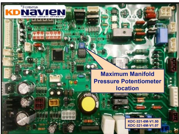
**Maximum Manifold Pressure Potentiometer location**
